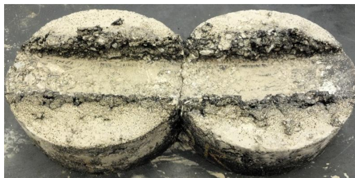
Figure 3.38: Test LW3 (64-22) specimens after testing
