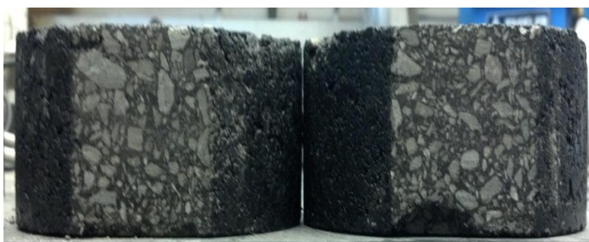
Figure 3.25: Test LW2 (PG 58-28) specimens before testing (side)
