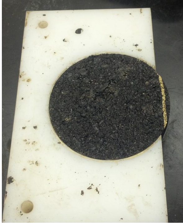
Figure A14: Marked core prepared to have 7.5 mm shaved off
