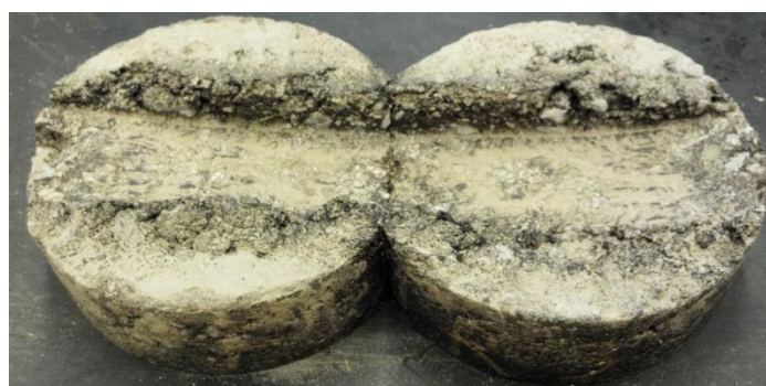
Figure 3.32: Test LH1 (64-22) specimens after testing (top)
