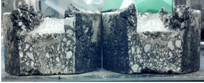
Figure 3.33: Test LH1 (64-22) specimens after testing (side)
