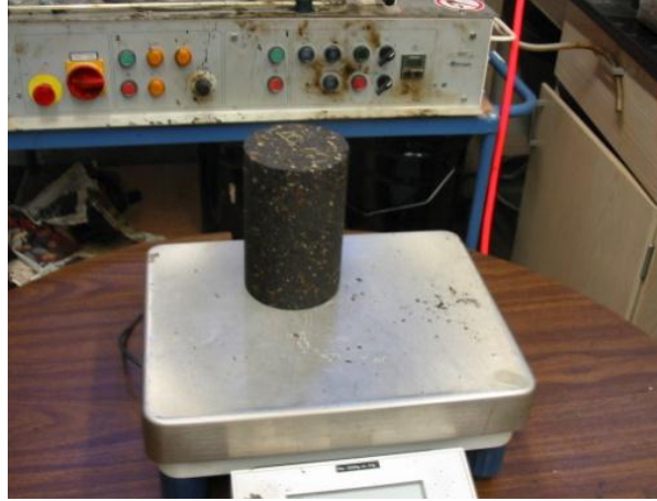
Figure A2: Weight of the sample in dry condition
