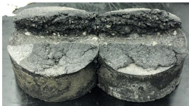
Figure 4.18: Test FH2 specimens after testing (top)
