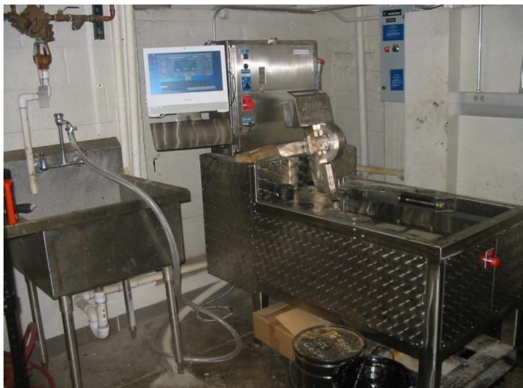
Figure 2.5: Hamburg Wheel Tracker Device
