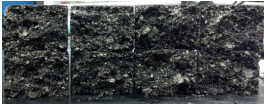
Figure 3.14: Stripping effects on lab mixed WMA specimens
