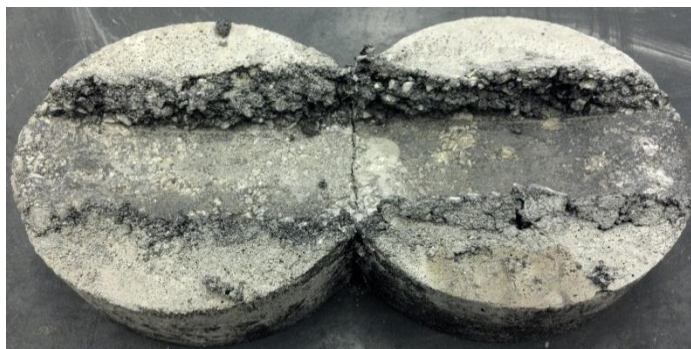
Figure 3.20: Test LH1 (PG 58-28) specimens after testing (top)
