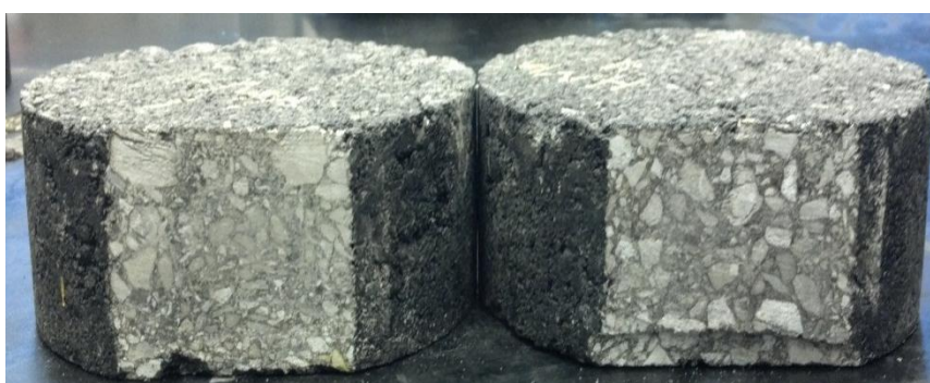
Figure 3.19: Test LH1 (PG 58-28) specimens before testing (side)
