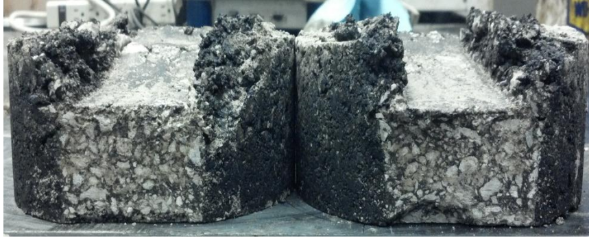
Figure 3.27: Test LW2 (PG 58-28) specimens after testing (side)
