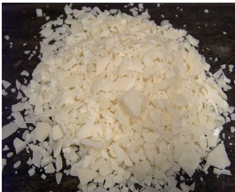
Figure 2.4: The Selected WMA Additive
