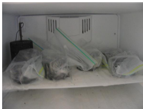
Figure A9: Freezing of the wet specimens at -18^{\circ}\text{C} for 16 hours
