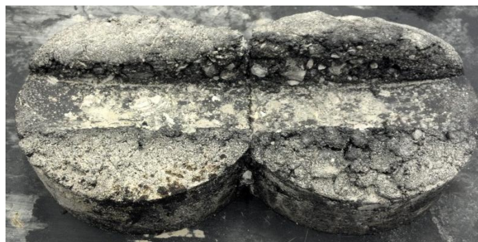
Figure 4.36: Test FWA3 specimens after testing (top)
