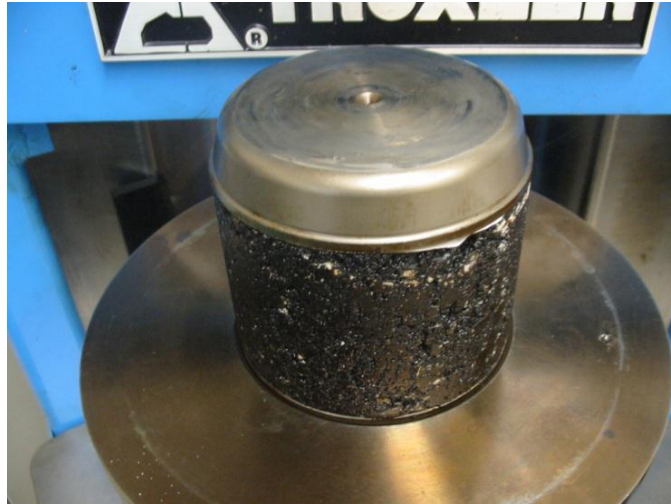
Figure A6: Specimen after compaction
