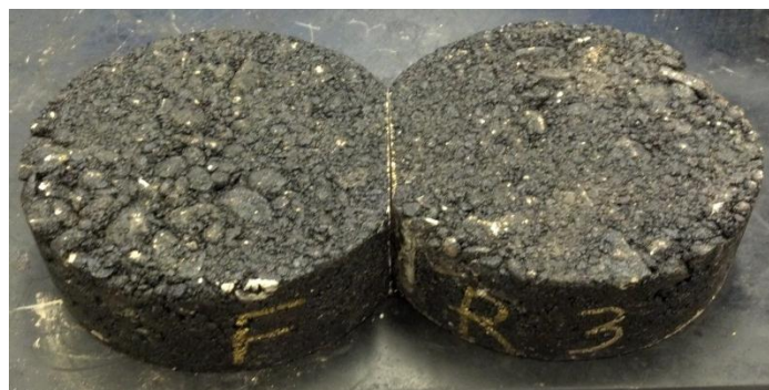
Figure 3.30: Test LH1 (64-22) specimens before testing (top)
