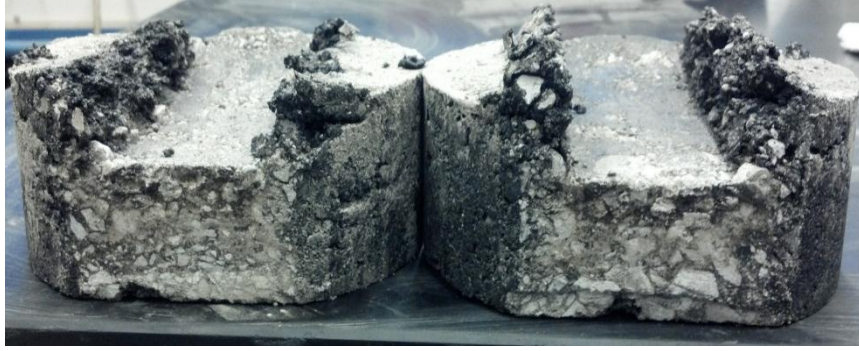
Figure 3.21: Test LH1 (PG 58-28) specimens after testing (side)
