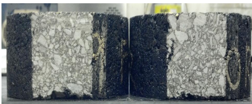
Figure 3.37: Test LW3 (64-22) specimens before testing
