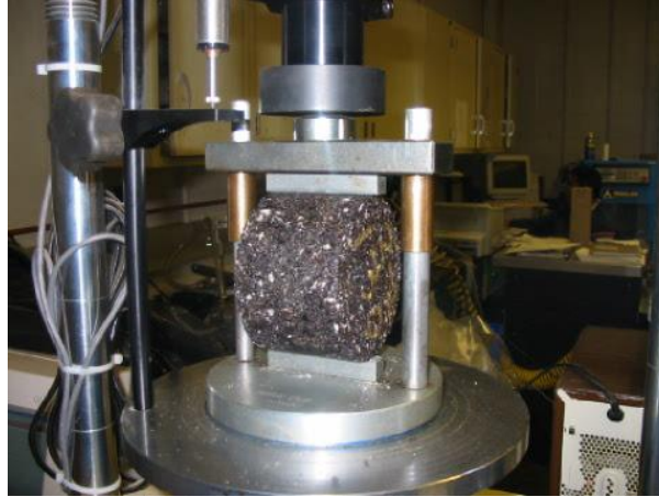
Figure A11: Indirect Tensile Strength of a specimen
