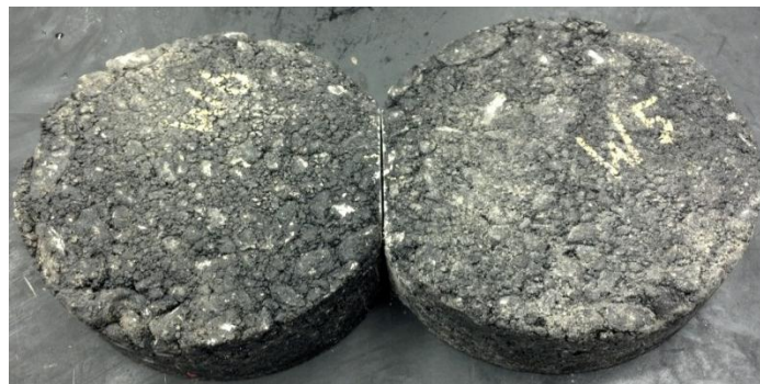
Figure 3.24: Test LW2 (PG 58-28) specimens before testing (top)
