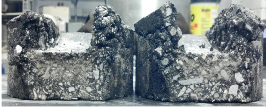
Figure 4.37: Test FWA3 specimens after testing (side)
