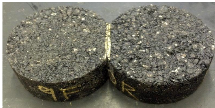
Figure 3.36: Test LW3 (64-22) specimens before testing
