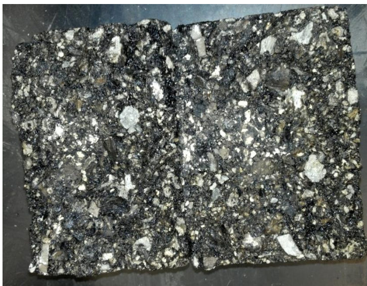
Figure 5.2: Stripping on a lab mixed WMA specimen
