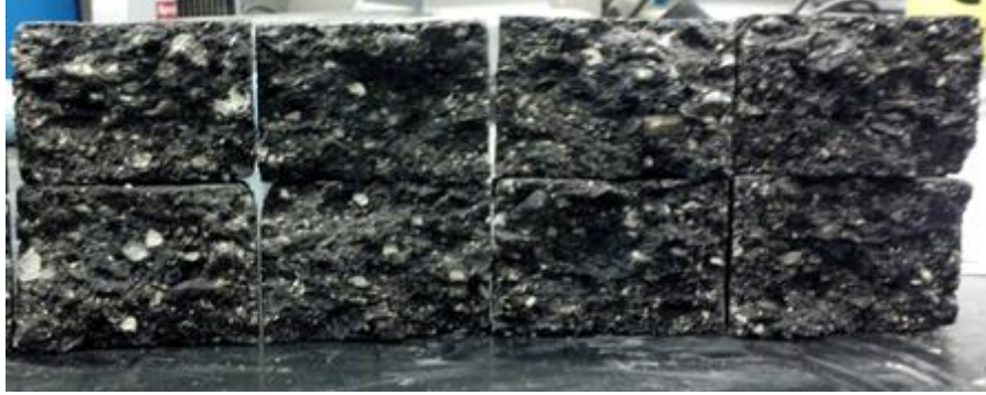
Figure 3.13: Stripping effects on lab mixed HMA specimens
