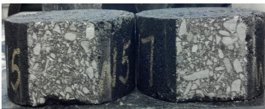
Figure 4.35: Test FWA3 specimens before testing (side)
