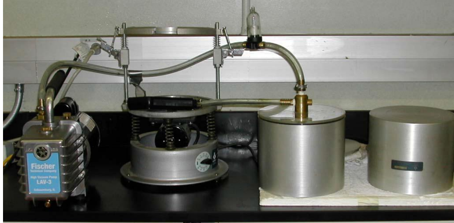
Figure A1: Rice specific gravity test equipment
